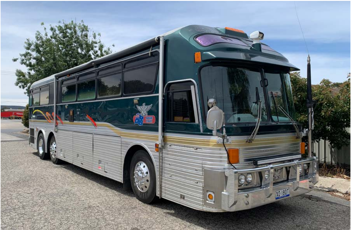
Spotted at Wimpy's Roadhouse Wodonga Vic. is this 1977 ex-Greyhound Silver Eagle express coach. Owner John said it has been retro-fitted with a 6V92T 2-stroke Detroit Diesel engine with a HT740 Allison Automatic. He plans to drive it all over Australia in the near future and recently fitted alloy wheels.
