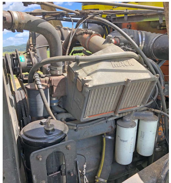
Mack's Tip Turbine 'CoolPower' air-to-air intercooling helps extract 285hp from the ENDT-676 Maxidyne engine.
