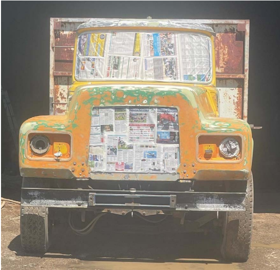
Cab restoration. Peter completed the rust repairs before a local spray painter applied the striking canary yellow and black colour scheme.
