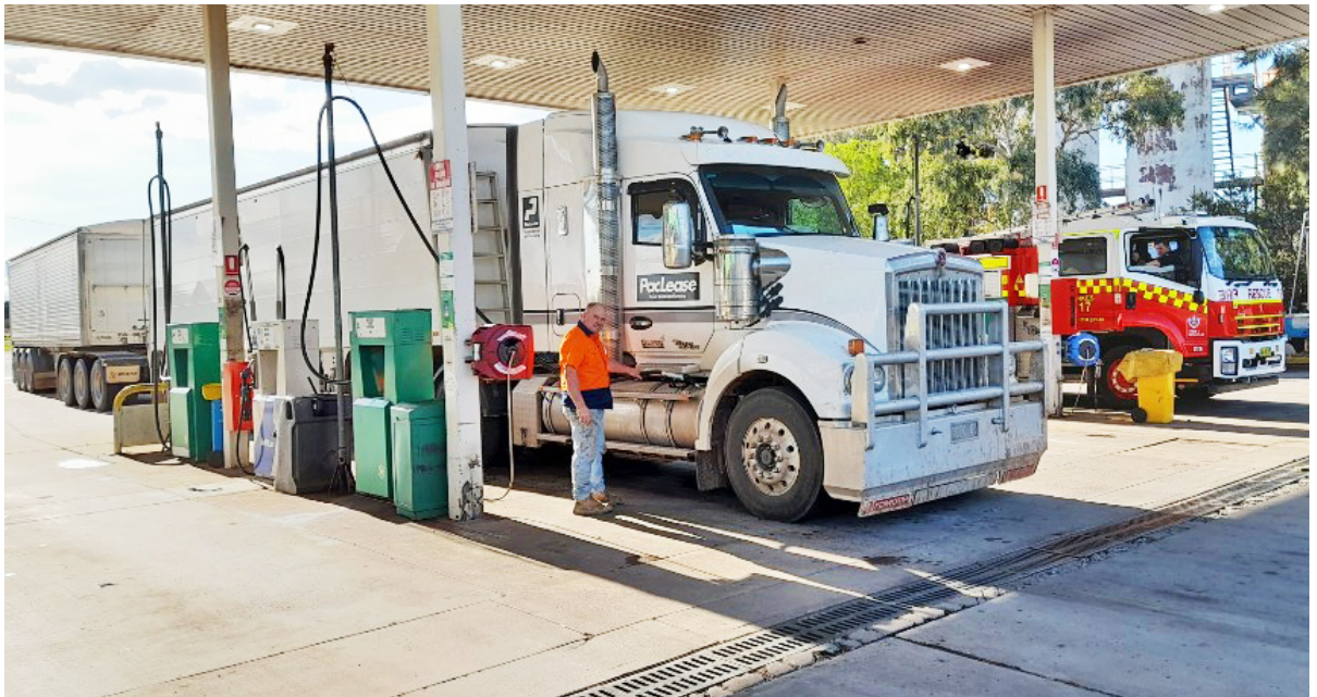
Road train, with centre delivery grain trailer (similar to a railway wagon) carting from Euabalong to Parkes grain sub terminal.
