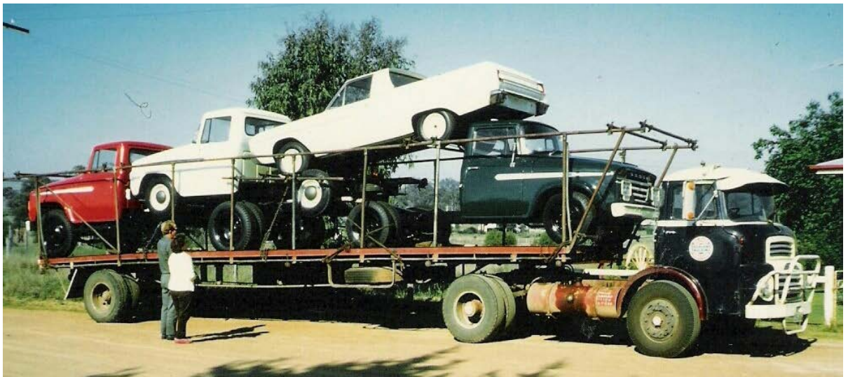
This photo was taken in 1968 outside my grandparents house in Warwick Qld. The truck is an Albion powered by a 6 cylinder Leyland 680 Super Power engine with a 6 speed over drive gearbox seen here with its single axle strap trailer. The Albion was owned by Overland Trucking that were based in Rocklea and the people in the photo looking at the new Dodge 7 series trucks and the new Valiant ute were my Dad, Ken Slade, & my grandmother, Celestine Stevens. Dad said that the Old Albion did a top speed of 46mph. Dad did Brisbane to Adelaide with General freight and returning with Chrysler vehicles and the round trip in 1968 usually took 10 days. — Shawn Slade
