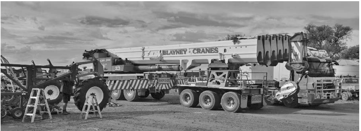
The mobile crane weighs 75t and is capable of lifting 220t
