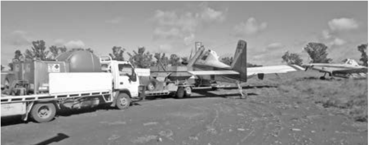
Loading Ag planes with urea to top dress wheat and barley to potentially increase the yield. This is usually done from the ground but planes were used because of all the rain and they take only 8 minutes per load. The trucks also carry Av-gas so the planes can be refuelled.
