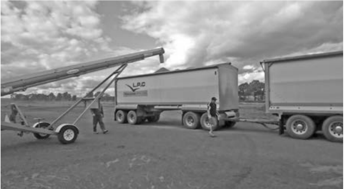
Loading Faba Beans (5-10 cents in size) by a flat bed auger so as to reduce cracking. The beans are transported to Melbourne to be manufactured into stock feed or put into a container and exported to Egypt. Photo by Annabelle Bonder .....
